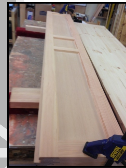
Manufacture of a replacement split leaf in our workshop.
